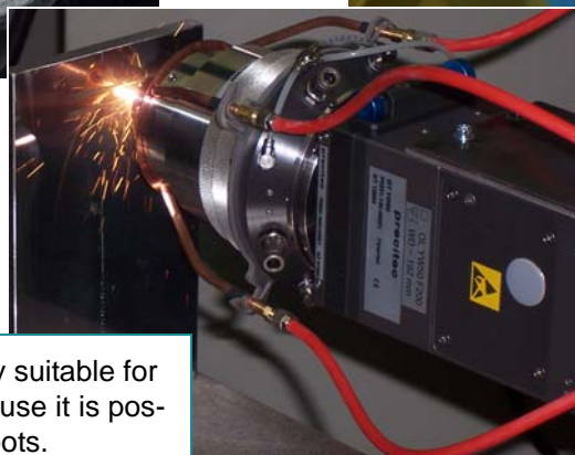
Radial cladding of valve seats
