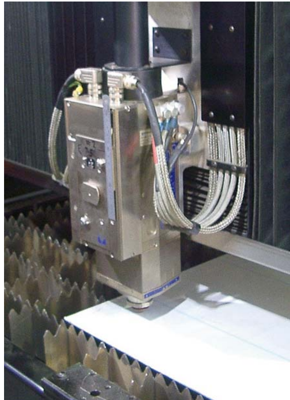
Laser cutting of coated, honey-comb-shaped aluminium sheets with 10" focal length
